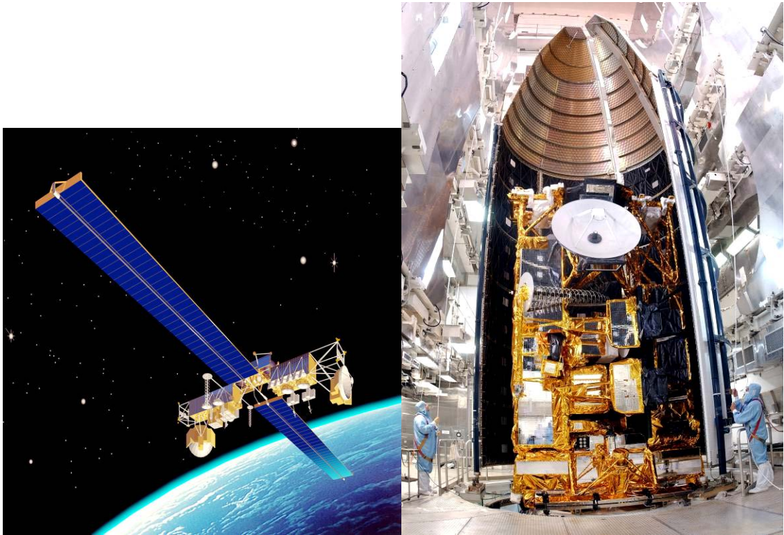
Left: An artist's concept depicts a Milstar II satellite in orbit. Right: The fifth Milstar satellite is enclosed in the payload fairing on top of its Titan IVB launch vehicle. Its successful launch on 15 January 2002 completed the operational constellation of four Milstar satellites. (Images courtesy Lockheed Martin Missiles and Space)
