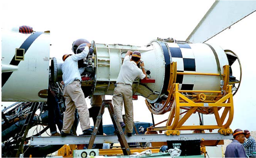
Top: Agena A spacecraft 1056 for Discoverer XIV is being integrated with Thor 237 before launch on 18 August 1960. Bottom left: The first Thor Agena launch vehicle sits on the pad at Vandenberg AFB before launching Discoverer I on 28 February 1959. Bottom right: The first Atlas Agena combination rises from the pad at Cape Canaveral in an unsuccessful attempt to launch MIDAS I on 26 February 1960. (U.S. Air Force photographs)
