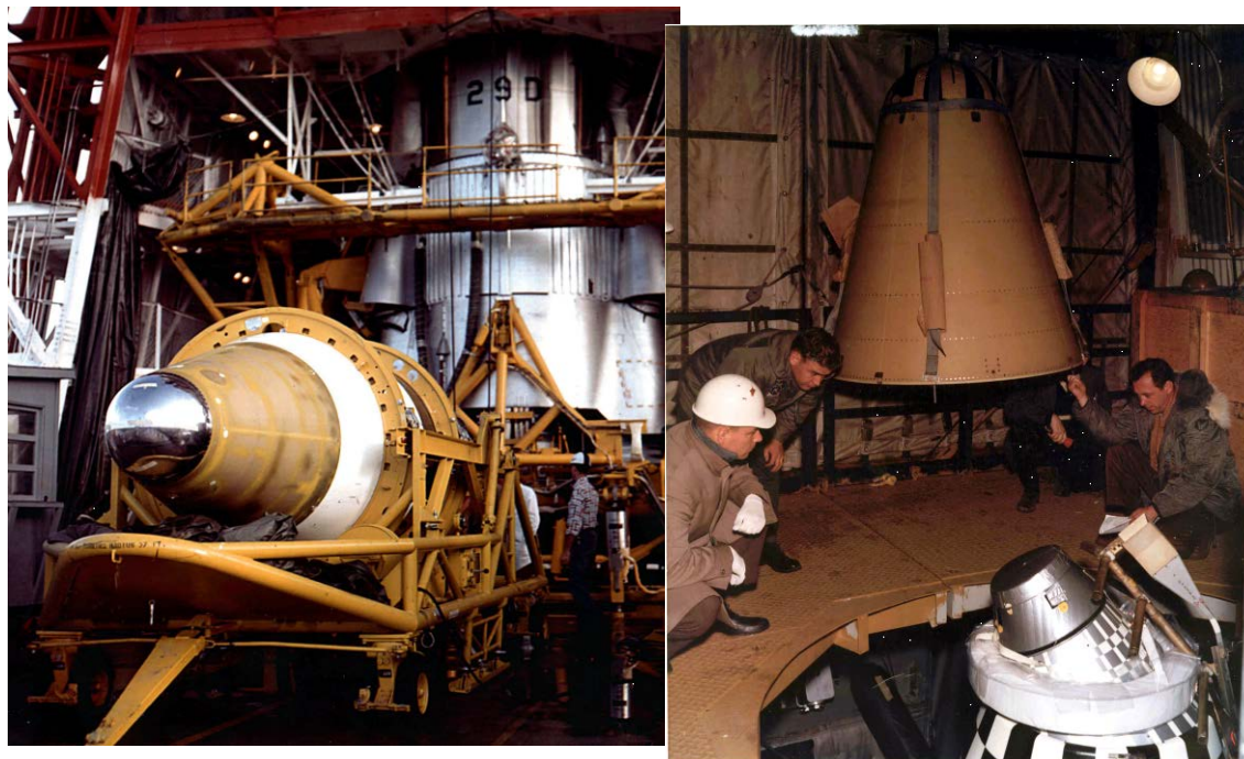
Left: The Agena spacecraft for MIDAS I waits for installation on Atlas 29D before its unsuccessful launch on 26 February 1960. Right: The payload for an advanced version of MIDAS, known as AFP 461, is covered with the Agena's nose cone before its unsuccessful launch as MIDAS 6 on 17 December 1962.
