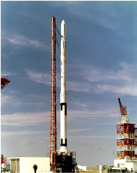
Left: A Blue Scout I (XRM-89) with a HETS payload sits on the pad at Cape Canaveral before its successful launch on 7 January 1961. Below: The HETS payload carrier being prepared for launch on a Blue Scout. (U.S. Air Force photographs)
